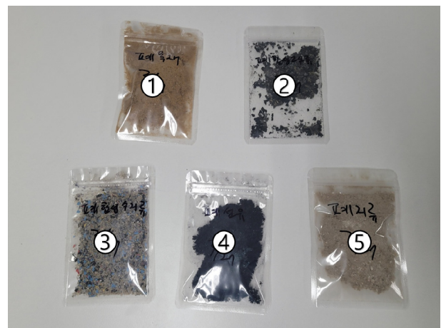
Fig. 1. Sample - ① Wood, ② Rubber, ③ Plastic, ④ Textile, ⑤ Paper
